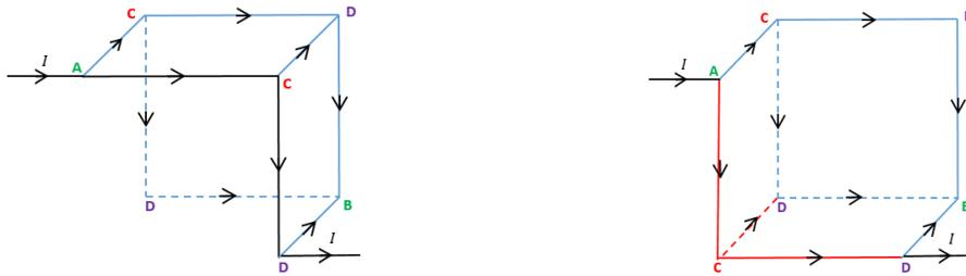
Due to symmetry, the junction "C" of resistors (2, 4, 5) and resistors (1, 8, 11) have the same potential ( $V_c$ ). So we can superimpose them like they are connected. In similar way, junctions "D" (7, 8, 9) and (5, 6, 10) have the same potential ( $V_D$ ).
