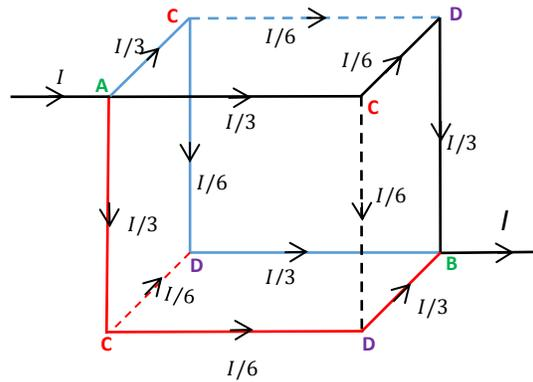
By applying Ohm's Law for the sum of the voltage in each path (series circuit):
