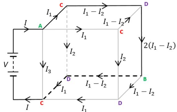
In addition the 2 longer paths “ACDCDC”, contribute the same way in configurations “1 and 3” also in “2 and 4”, therefore we can say calculation for the two main paths are all similar due to symmetry. So we proceed and treat them the same way.
