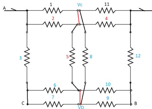
As can be seen in the diagram above the 2 points C, in the same face with the same potential are connected with a red line, same way for points D, now we need to simplify parallel resistors in the circuit. Given all the resistors are equal to R:
