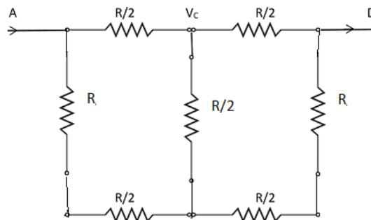
Now apply star (Y) to triangle ( $\Delta$ ) transformation for the 3 central resistors R/2 on top:
